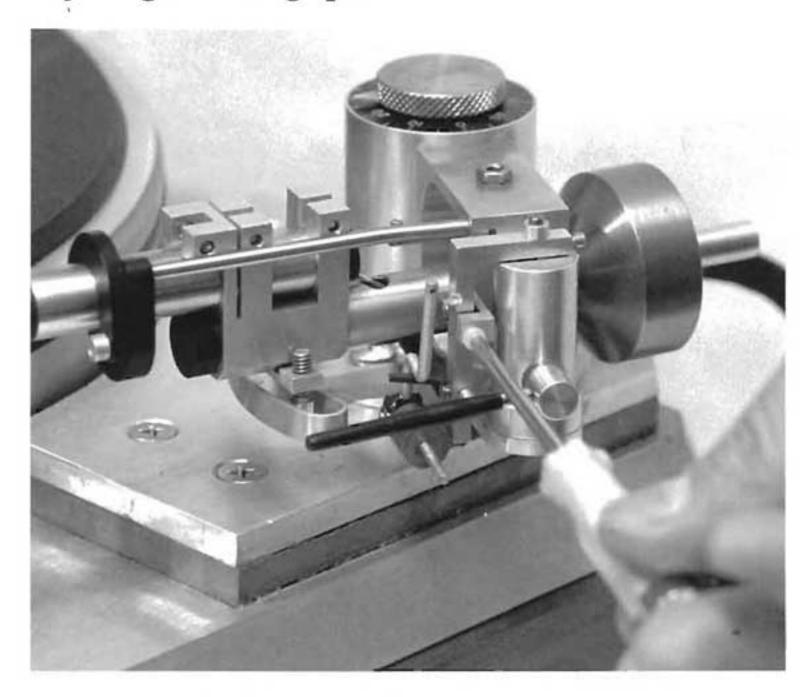
Use the cueing-device lever to raise the tone arm, and move the tone arm to a position above the record's surface.
