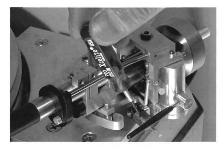
Place the cartridge alignment gauge on the platter. Point sight line at tonearm pivot point.
