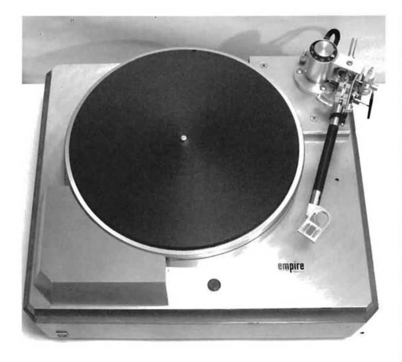
Before drilling, check placement. Remove the jig from the spindle, place the tone arm on the armboard and line up the mounting-screw holes with the hole marks. If your turntable has a cover, check to be sure it can be lowered over the tone arm.
