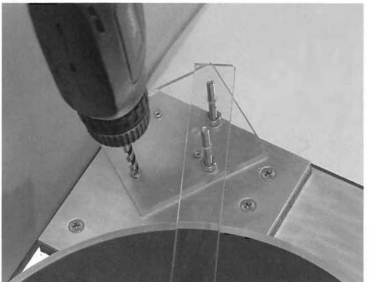
If satisfied with placement, replace the jig on the spindle, and drill holes.
