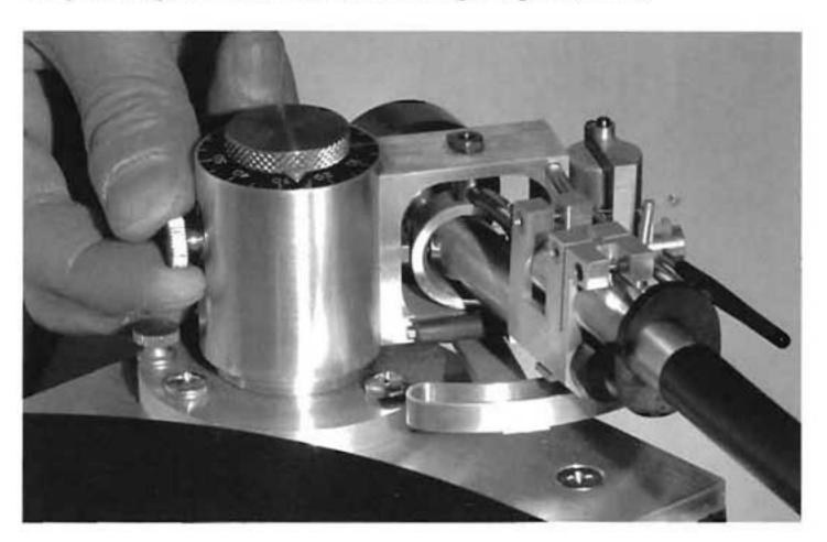
Loosen then lightly re-tighten the VTA locking screw on the side of the VTA tower.
