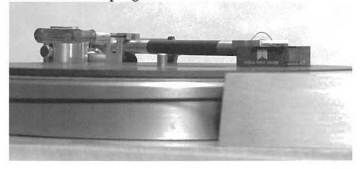
Use the P21 Allen wrench on the azimuth adjustment screw (below), turning it until the head shell becomes parallel to the platter, using the stylus force gauge as your straight edge. (Clockwise lowers the right edge, counter-clockwise lowers the left edge.)
