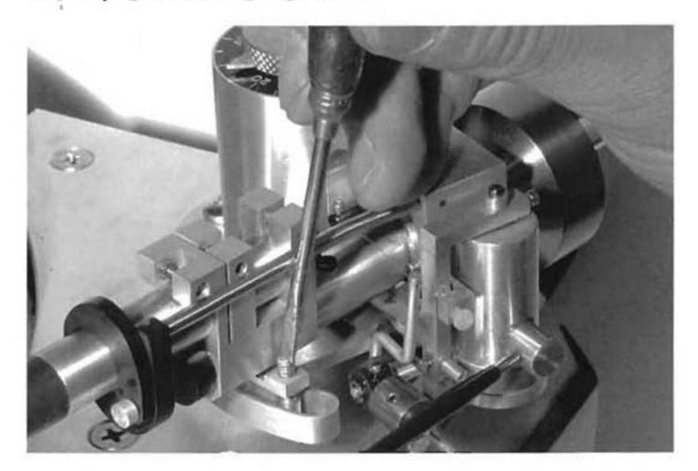
Turn the screw on top of the damping trough to adjust damping (clockwise to lower the screw, counter-clockwise to raise).
