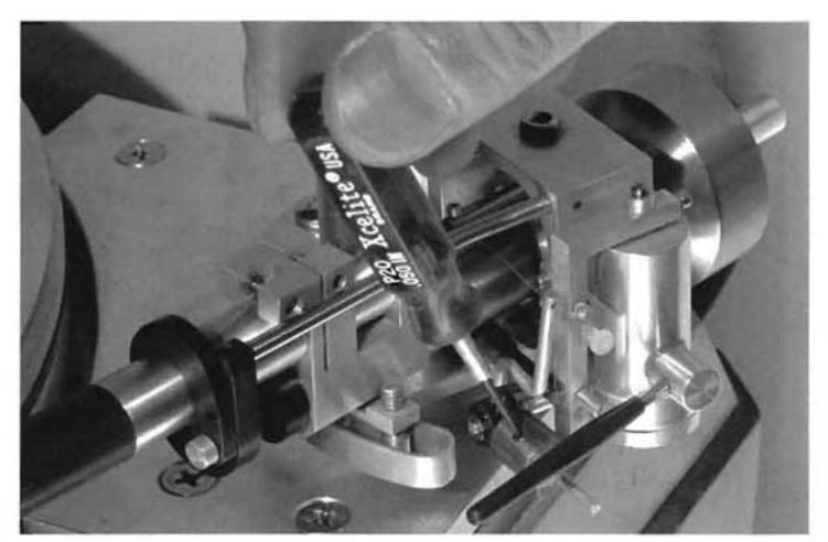
Use the P20 (0.50") Allen wrench to loosen the anti-skate weight screw.
